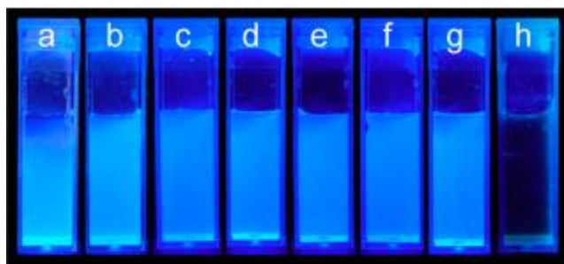
Figure 4. Response of Ur-MOF aqueous dispersions (1 mg in 2 mL water) toward the additions of various nitro analyte aqueous solutions (200 \mu L each) under UV light ( \lambda_{max} = 365 nm) (a = TNT, b = NM, c = RDX, d = 2,4-DNT, e = 2,6-DNT, f = NB, g = DMNB, h = TNP).
