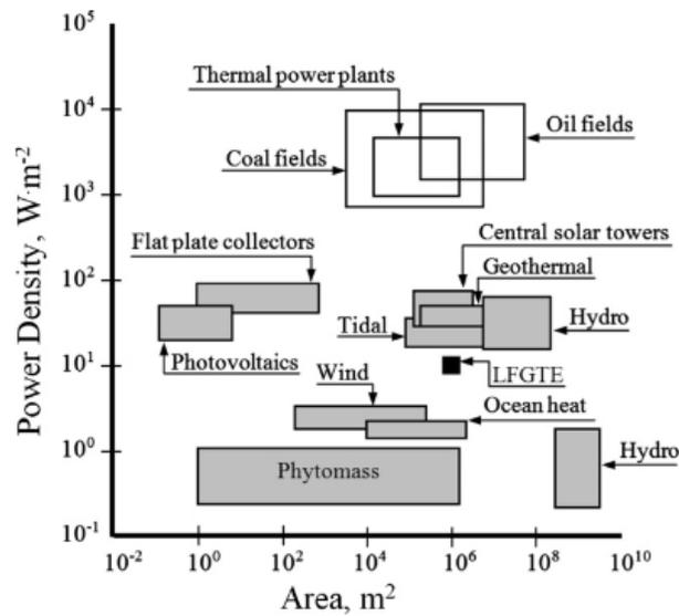
Fig. 4. Power density of LFGTE in comparison to other energy sources.<sup>13</sup>
